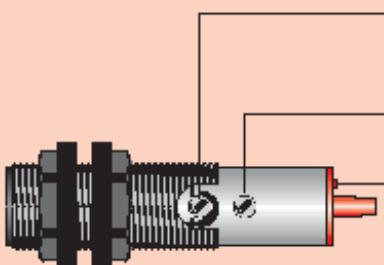
● **TRIMMER FOR THE SENSING RANGE ADJUSTMENT:** The photocell is supplied with max. sensing range with the trimmer totally rotated in the clockwise direction. The sensitivity reduces by rotating the trimmer in the anti-clockwise direction.
