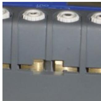
Connect your probes by simply pushing on the terminal top and insert wires of up to 3 mm or 10 AWG diameter and compensated thermocouple connectors.
