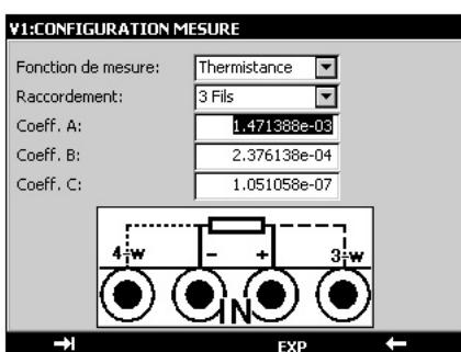
With 50 Kohms range and Steinhart – Hart equation integrated, thermistors can be entered into CALYS 150 and tested. Steinhart-hart equation is as follows:  $1 = A + B(\ln(R)) + C(\ln(R))^3 T$  Where: A, B and C are usually calculated according to temperature at 0°C, 25°C and 70°C
