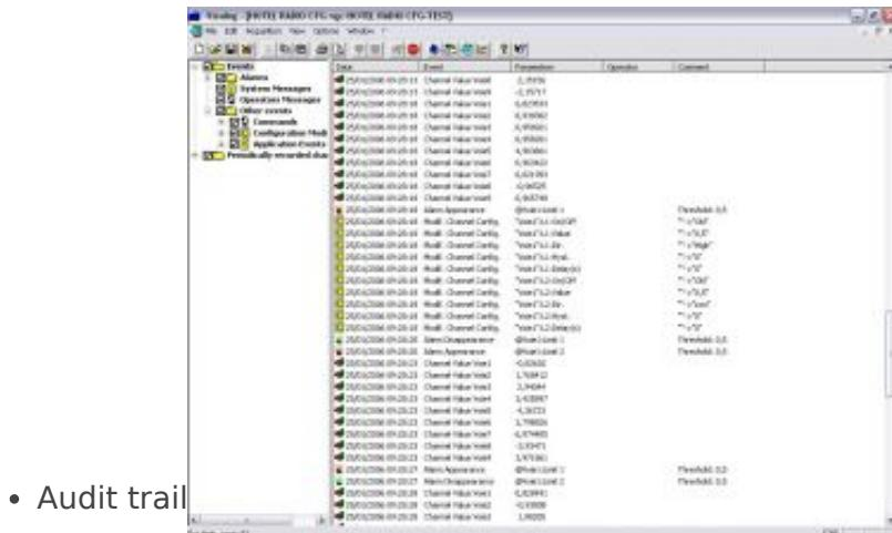
All the events are recorded into a protected file: connections, disconnections, alarms appearance/clearance, configuration modifications, results readings...
