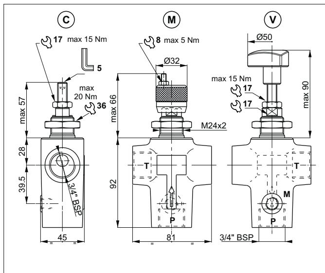
The direct acting relief valve with CMP30 cartridge limits the pressure in the hydraulic circuit.
