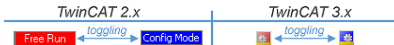
Fig. 192: Displaying of “Free Run” and “Config Mode” toggling right below in the status bar
