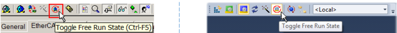
Fig. 193: TwinCAT can also be switched to this state by using a button (left: TwinCAT 2; right: TwinCAT 3)
