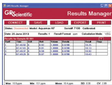
This is a windows application that allows you to view and print sets of results created by the Aquamax KF Coulometric. It can download results directly from the titrator through a serial port connection, or open result files
