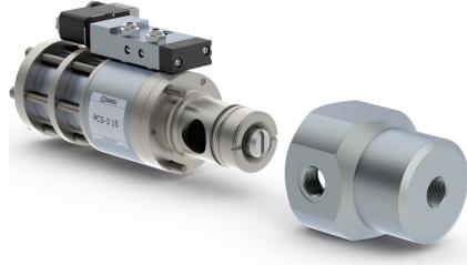
**2/2 way valve** externally controlled**pressure range** PN 0-200 bar**orifice** DN 15 mm**connection** thread/cartridge**function** valve
