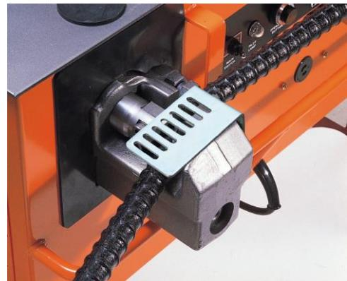
**Cutter and bender combo in one compact unit.**
