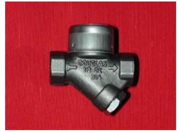
Reduced dimension and weight simple and reliable. It discharges air. It withstands waterhammer. Condensate discharge is intermittent. Some loss of live steam.
