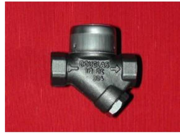
Reduced dimension and weight simple and reliable. **Special air venting disc.** It withstands waterhammer. Condensate discharge is intermittent. Some loss of live steam.
