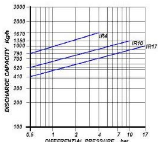
Cold water capacities are 2 to 4 times greater than the above . Safety factor = 1.2 – 1.5
