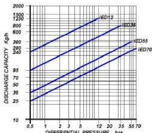
Cold water capacities are 2 to 4 times greater than the above . Safety factor = 1.2 – 1.5
