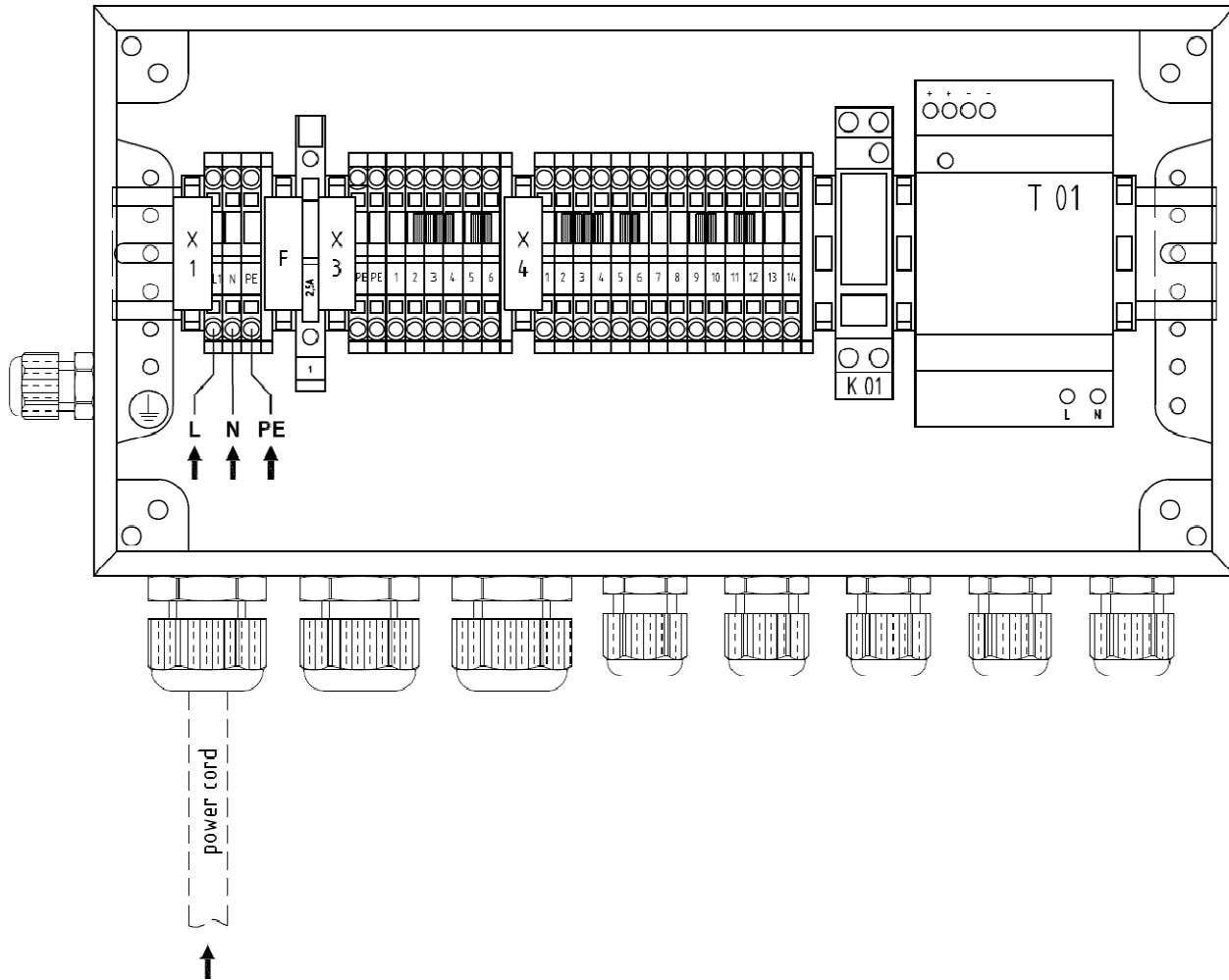
Fig. 12 Terminal connection diagram Digox 601 dac: power supply connection left-hand side up to S/N 681xxxxxx00038
