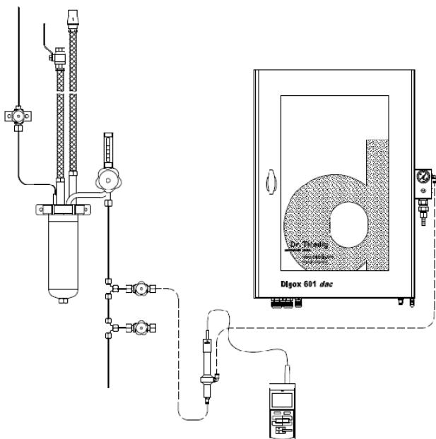
Fig. 55 Measurement arrangement for specific conductivity SC in series
