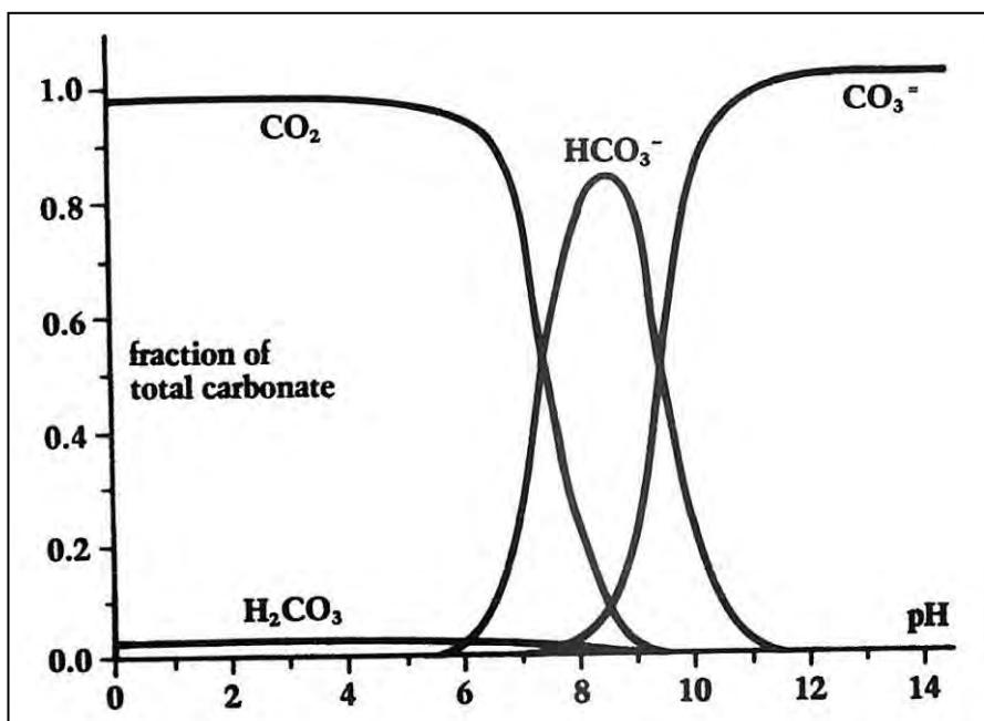
Fig. 3 Regression curve for dissolved carbon dioxide
