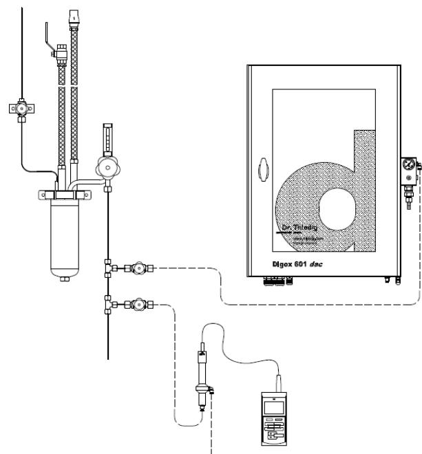
Fig. 56 Measurement arrangement for specific conductivity SC parallel to the device
