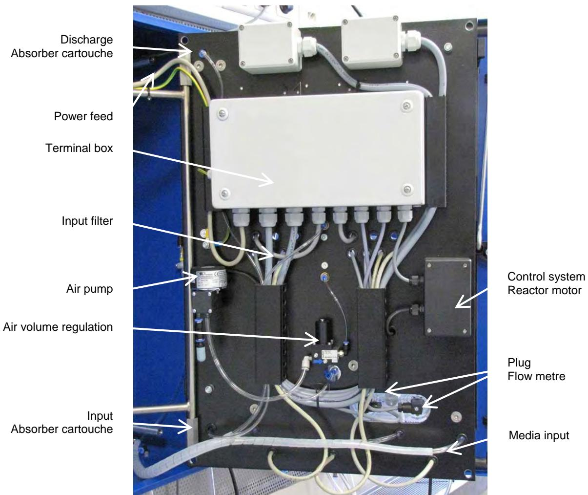
Fig. 10 Digox 601 dac folded out
