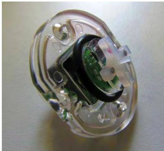
Fig. 43 Dismantled flow metre with seal
