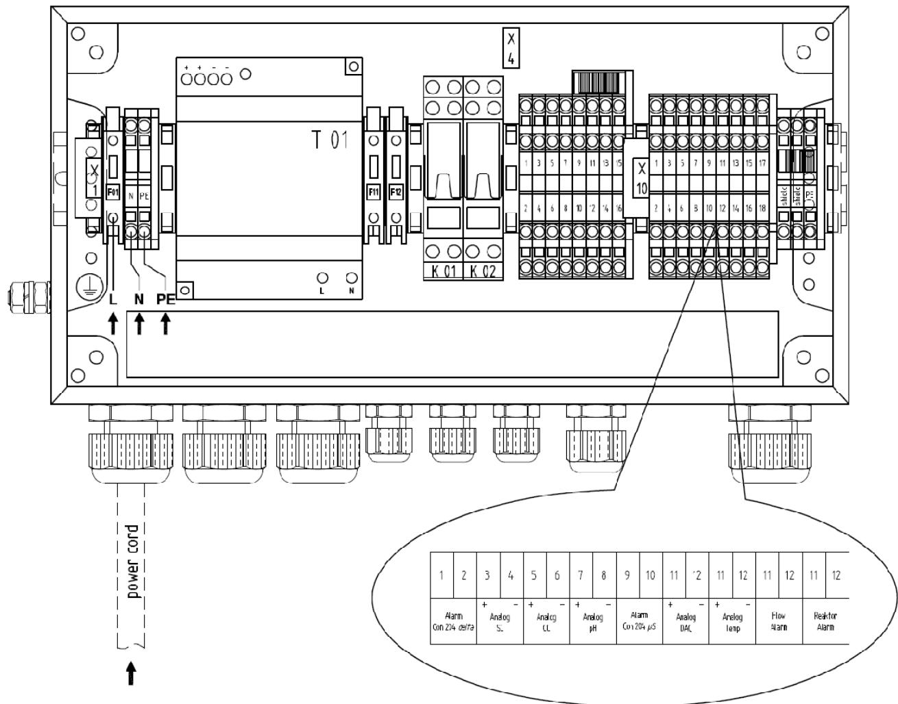
Fig. 15 Terminal connection diagram Digox 601 dac: power supply connection left-hand side from S/N 681xxxxx00039
