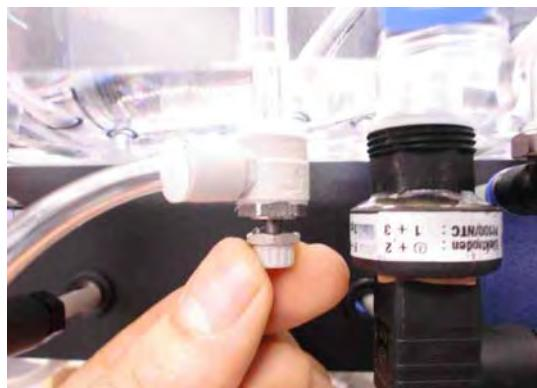
Fig. 39 Opening the valve for comparison measurements
