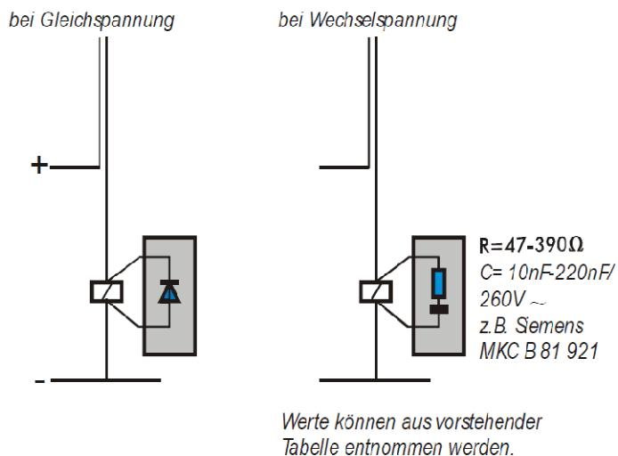
Fig. 11 Relay switching under direct or alternating voltage
