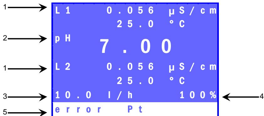
Fig. 20 Con 204 *delta* display with possible visualisations
