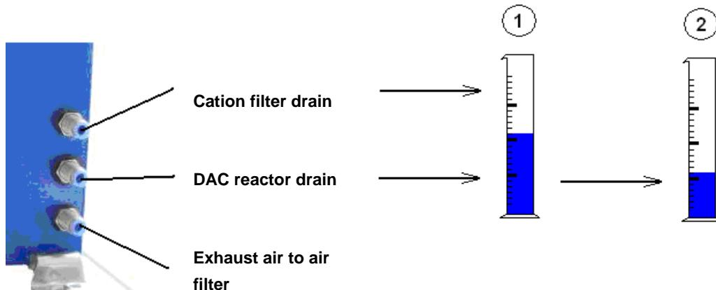
Fig. 42 Measurement arrangement for determining real flow rate
