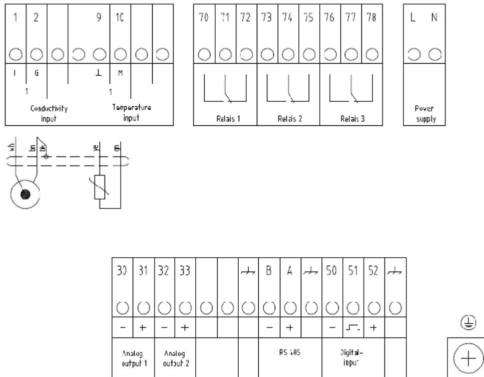
Fig. 19 Terminal connection plan Con 204  $\mu$ S
