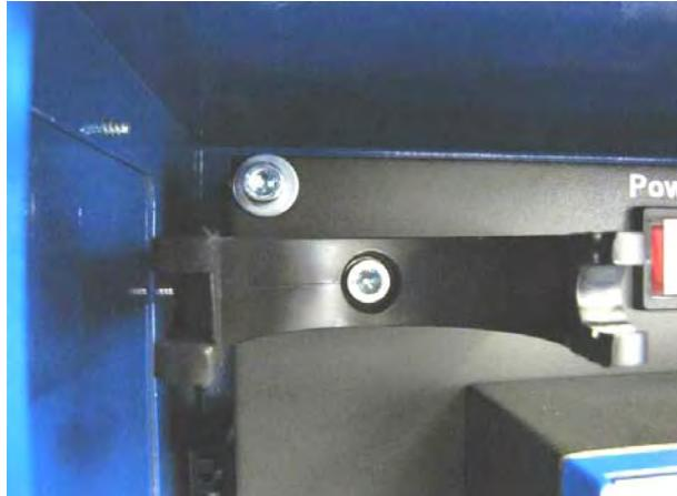
Fig. 5 Example of location of top left retaining screw
