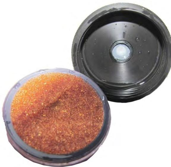
Fig. 51 Dismantled cartouche cover with seal
