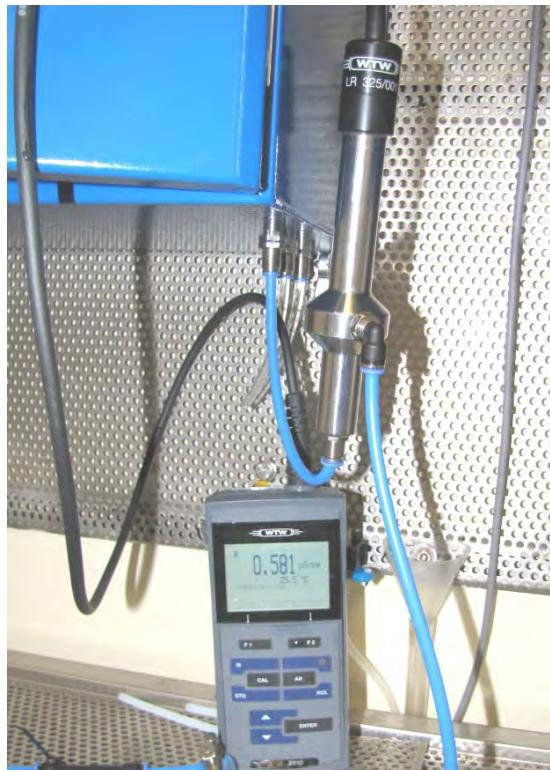
Fig. 57 Measuring arrangement cation conductivity CC
