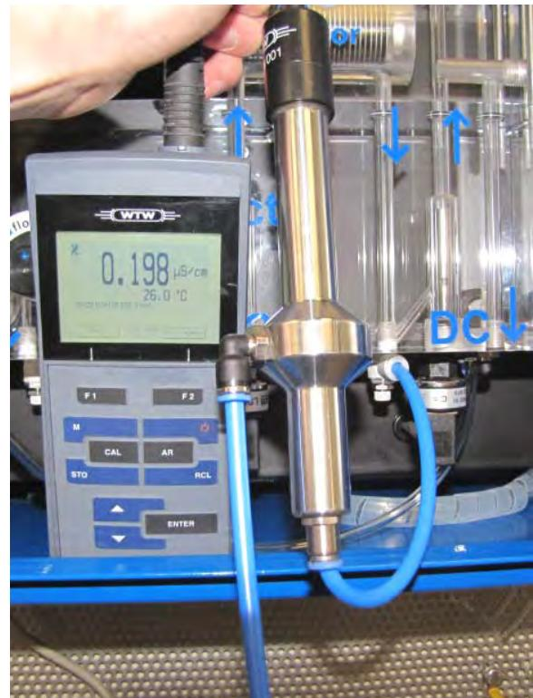
Fig. 58 Measuring arrangement degassed conductivity DG
