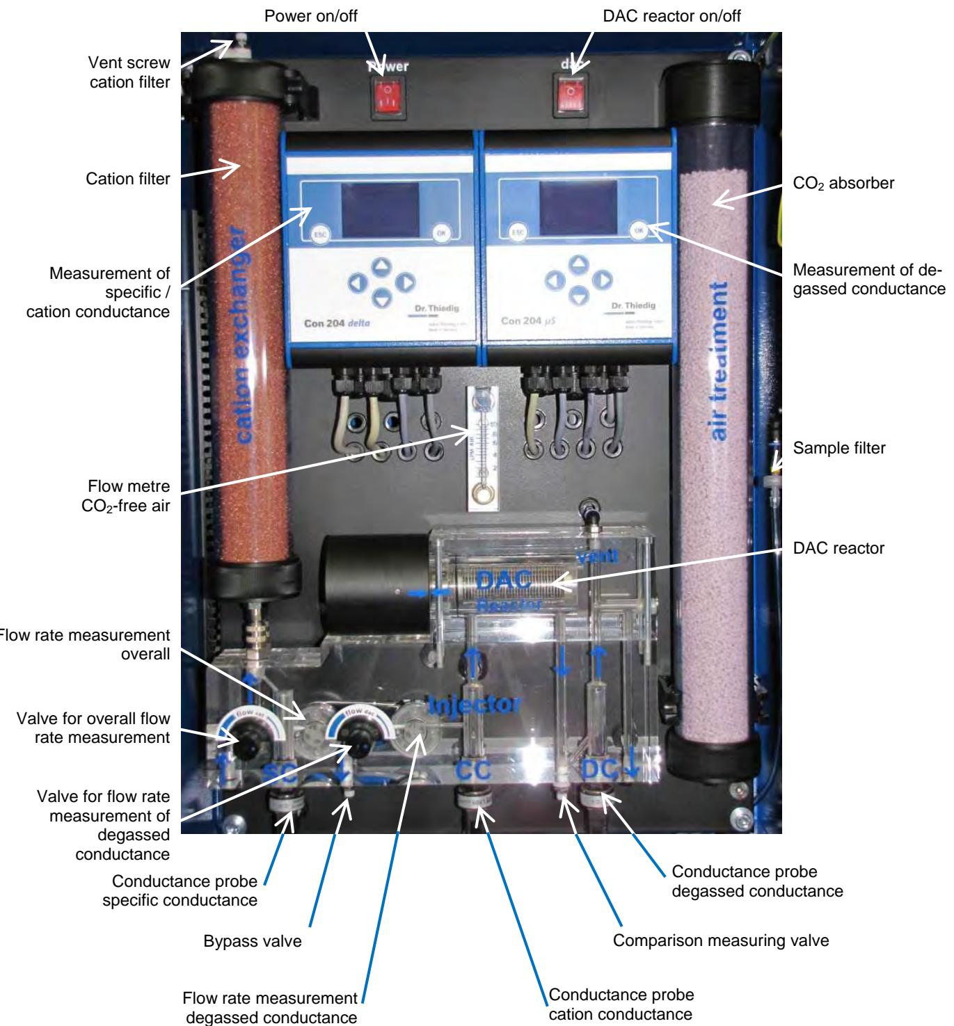
Fig. 23 DAC analyser with cation exchanger, DAC reactor, CO<sub>2</sub> absorber and operating elements
