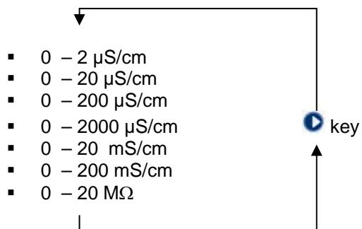
The required measuring range must be confirmed using the OK key and will then be applied to "Measuring range" (lines 3 and 4).
