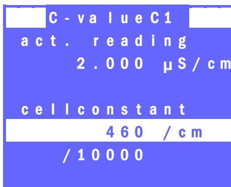
Fig. 28 screen for setting the cell constant.
