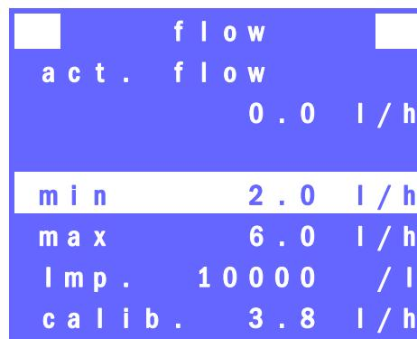
Fig. 41 Display with flow rate settings on the Con 204  $\mu\text{S}$
