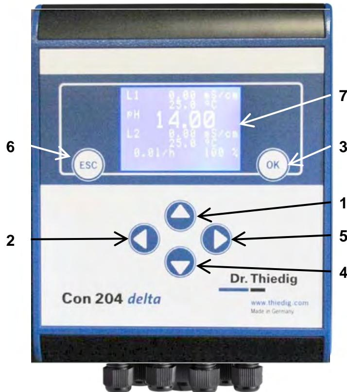
The Con 204 *delta* conductivity measuring amplifier is operated using a 6-key membrane keypad.
