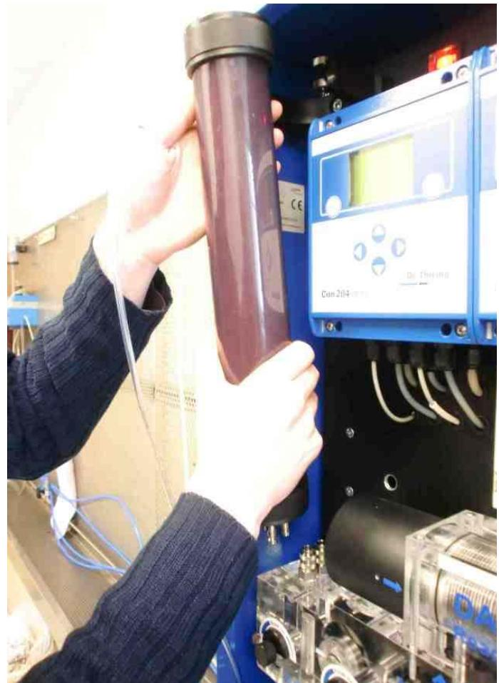
Fig. 47 Removing the cartouche
