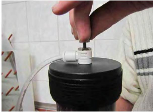
Fig. 48 Opening the air bleed valve
