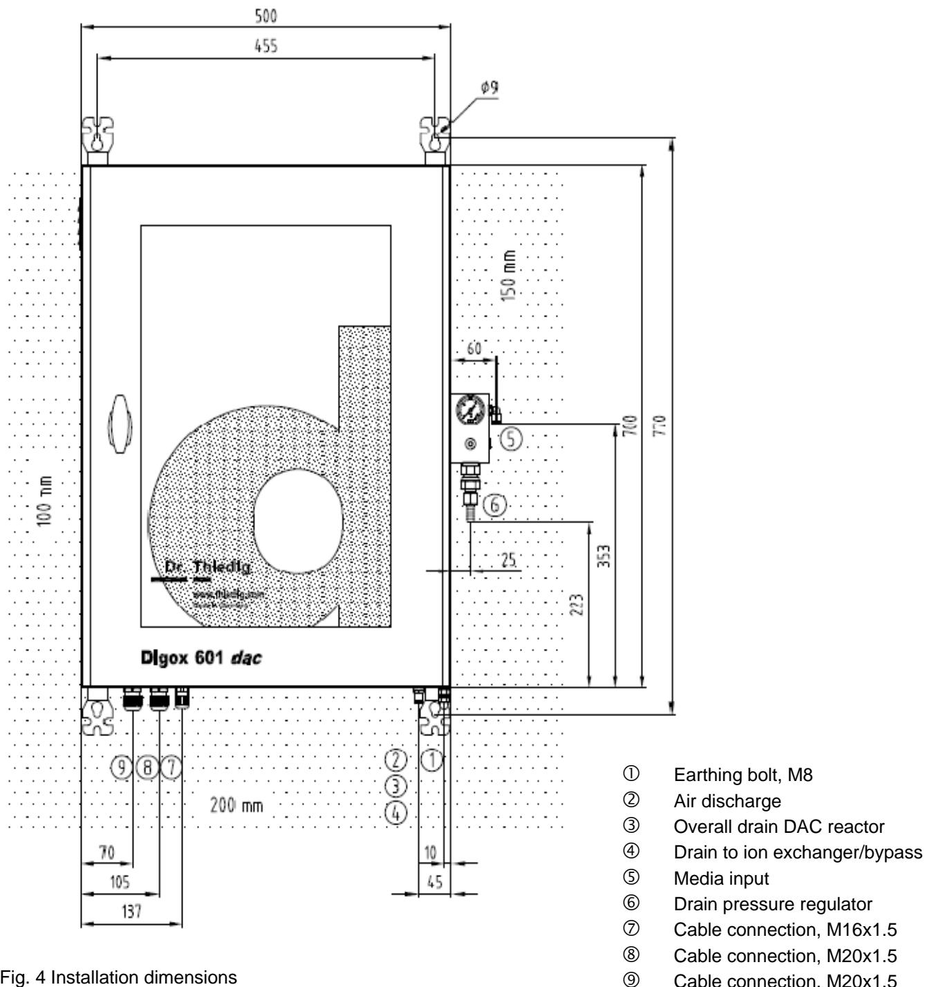
Fig. 4 Installation dimensions
