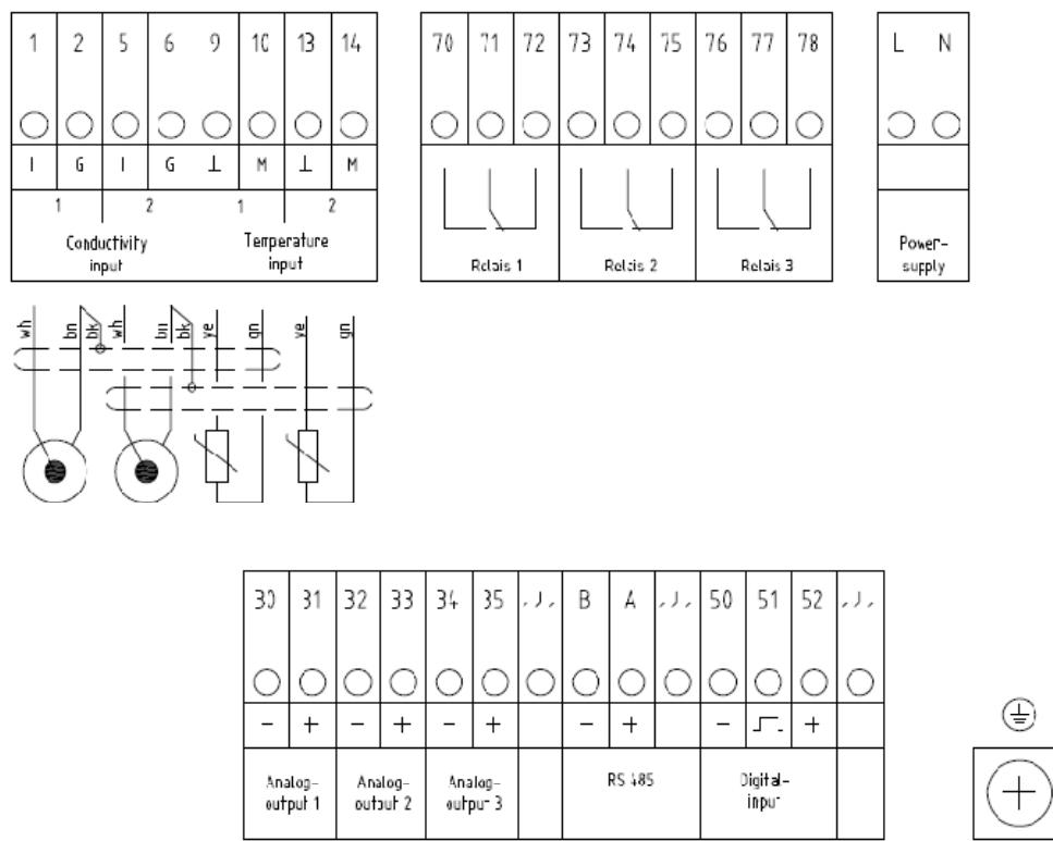
Fig. 18 Terminal connection plan Con 204 *delta*
