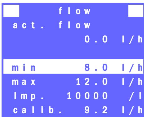
Fig. 40 Display with flow rate settings on the Con 204 *delta*
