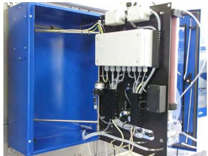
Fig. 6 Swivel frame pulled out
