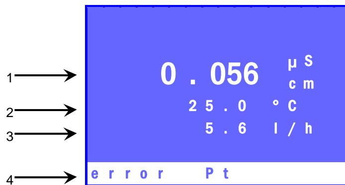
Fig. 21 Con 204  $\mu$ S display with possible visualisations
