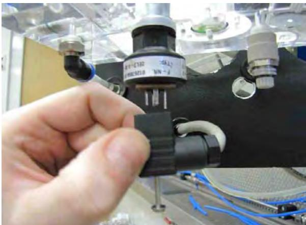
Fig. 37 Removing sensor plugs
