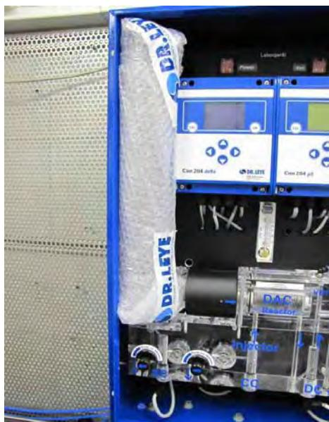
Fig. 62 Separately packed ion exchanger cartouche placed in container
