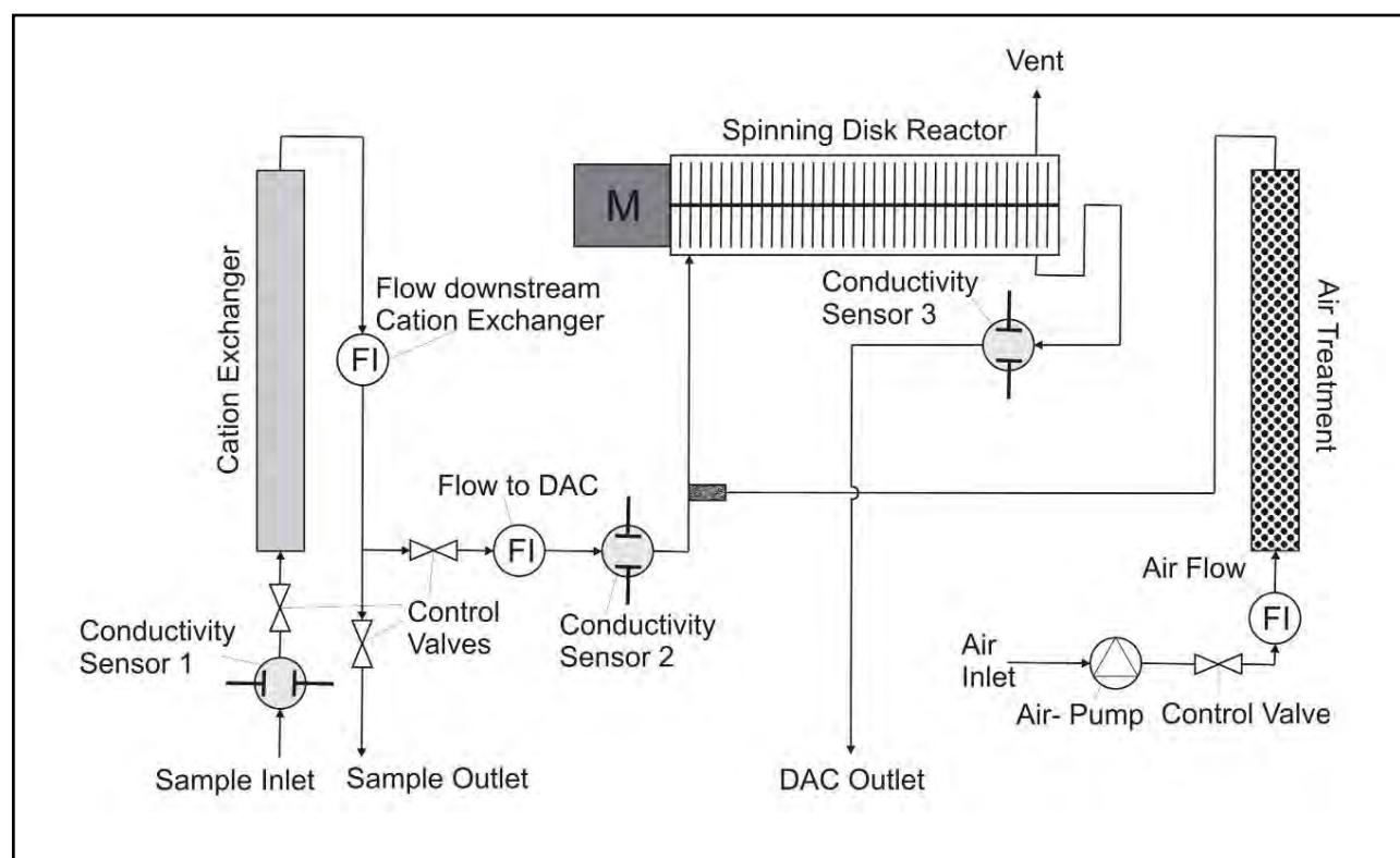
Fig. 2 Schematic setup of complete DAC measuring instrument
