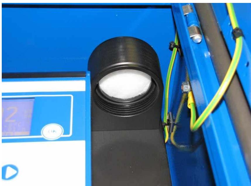
Fig. 54 Upper section, filter and seal
