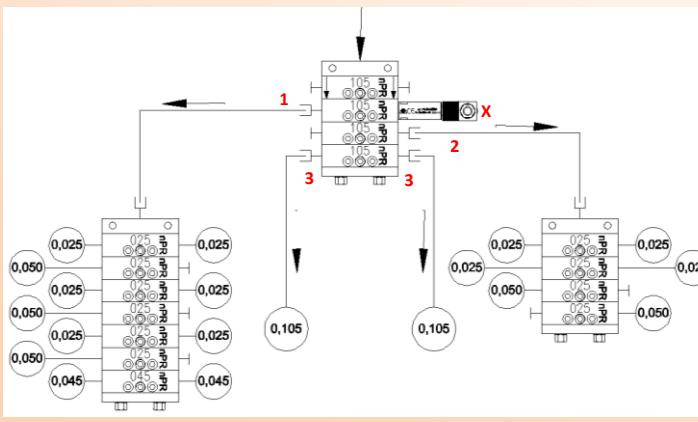
The master divider element nPr105 (1) controls a group of 6 divider elements with a flow rate of 0.025cm<sup>3</sup>/cycle and one with 0.045 cm<sup>3</sup>/cycle.
