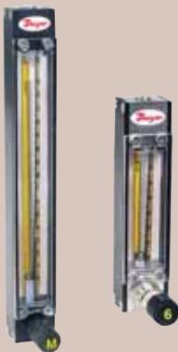
Panel Mounting: Drill two 5/8" dia. holes at 4.5" apart for 65 mm models and 8.812" apart for 150 mm models (center-to center).
