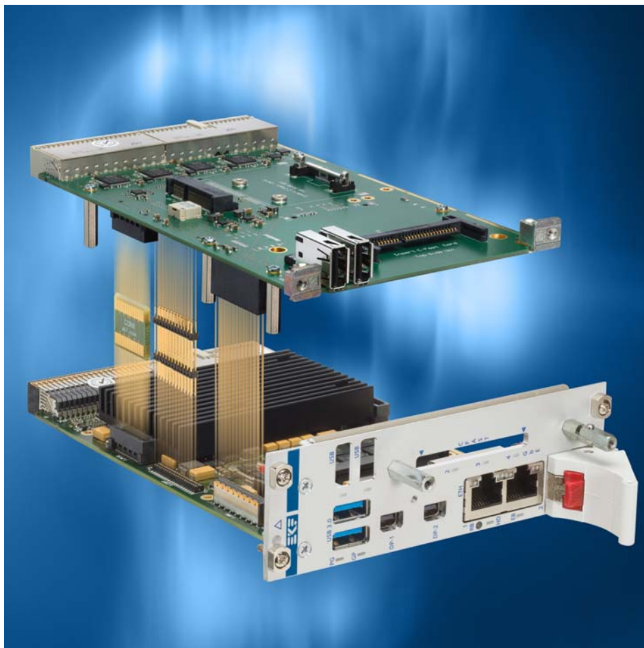
Expansion Interface Connectors for 8HP Mezzanine Assembly
