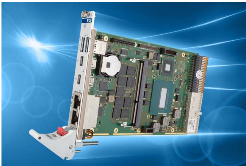
PC4-PRESTO (Heatsink & SO-DIMM Removed)
