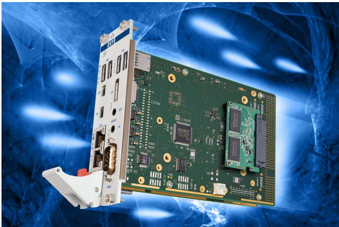
PC4-PRESTO w. PCS-BALLET Side Card 8HP Assembly (Slim SATA SSD)
