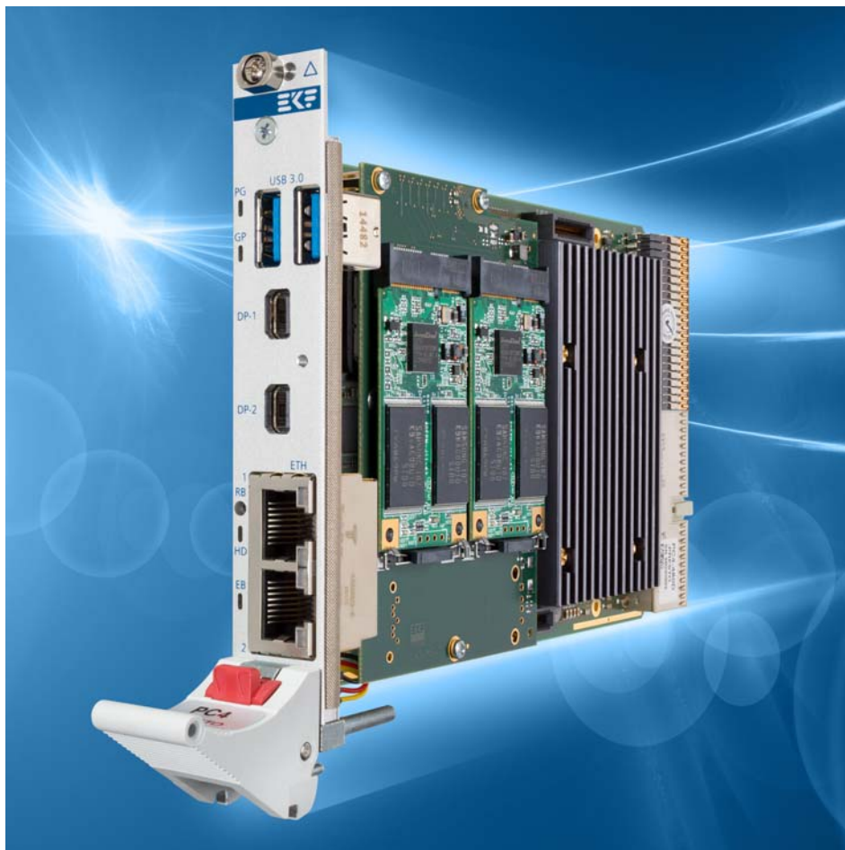
PC4-PRESTO w. C47-MSATA Dual-SSD Mezzanine Storage Module
