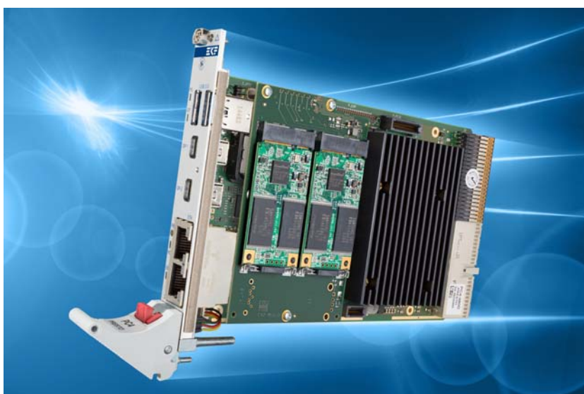
PC4-PRESTO w. Low Profile mSATA SSD Mezzanine
