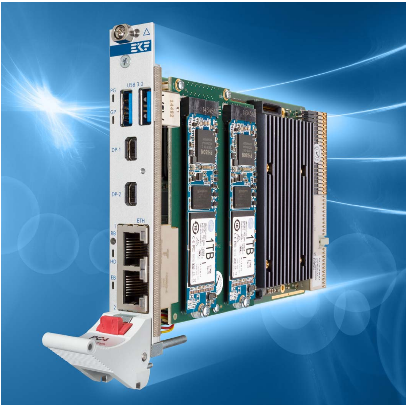
PC4-PRESTO w. C48-M2 Low Profile SSD Mass-Storage Mezzanine Module 4HP Assembly
