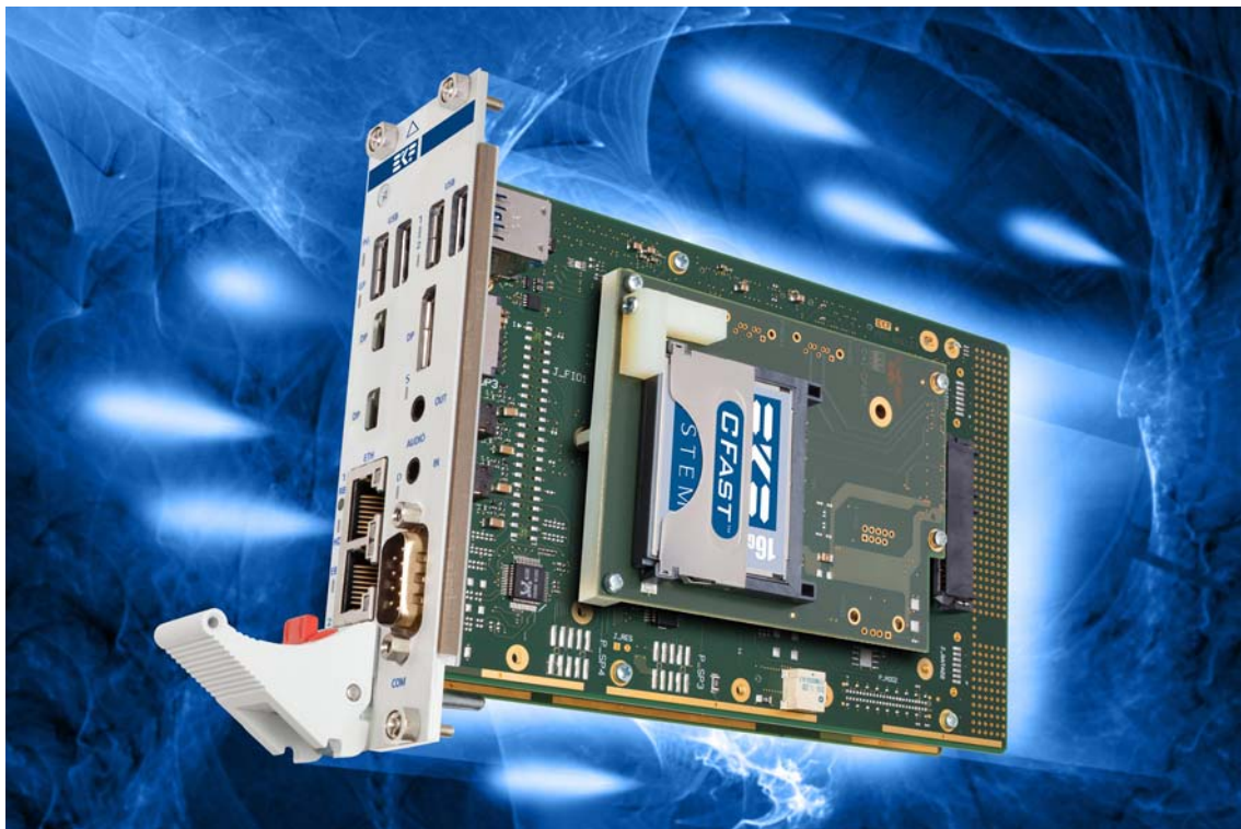
PC4-PRESTO w. PCS-BALLET Side Card 8HP Assembly (CFAST SSD)
