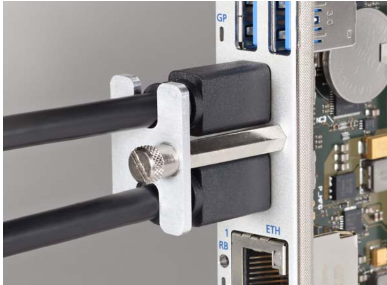
Option Screw-Lock Plate for mDP Cable Connectors
