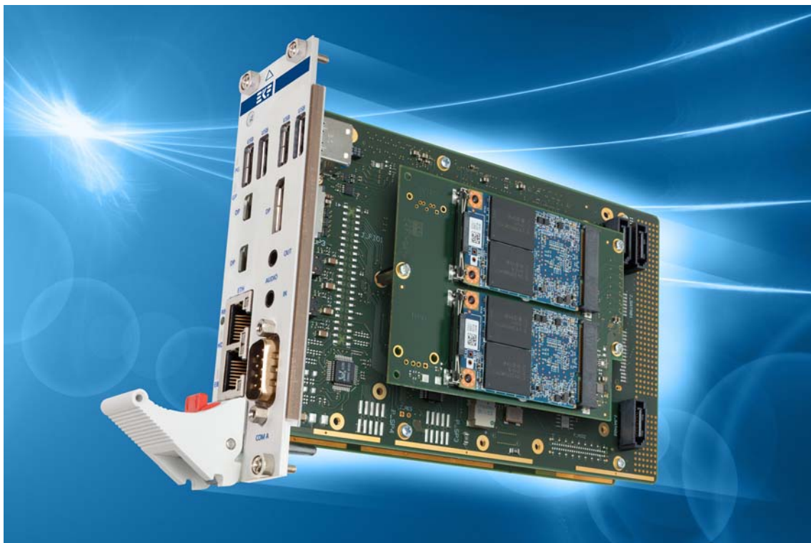
PC4-PRESTO w. PCS-BALLET Side Card 8HP Assembly (Dual mSATA SSD)
