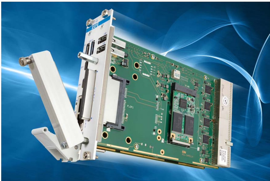
PC4-PRESTO w. PCL-CAPELLA Side Card 8HP Assembly
