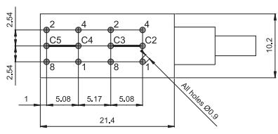
Commons (C2, C3) must be connected together on the PCB
