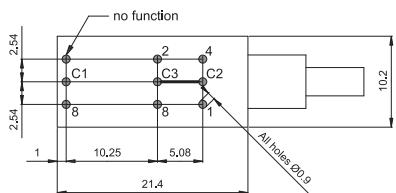
Commons (C2, C3) must be connected together on the PCB
