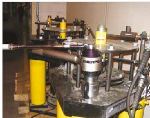
◀ Enerpac Reaction Bar Torque Multiplier E393 used to manually torque bolts up to 3170 Ft.lbs
