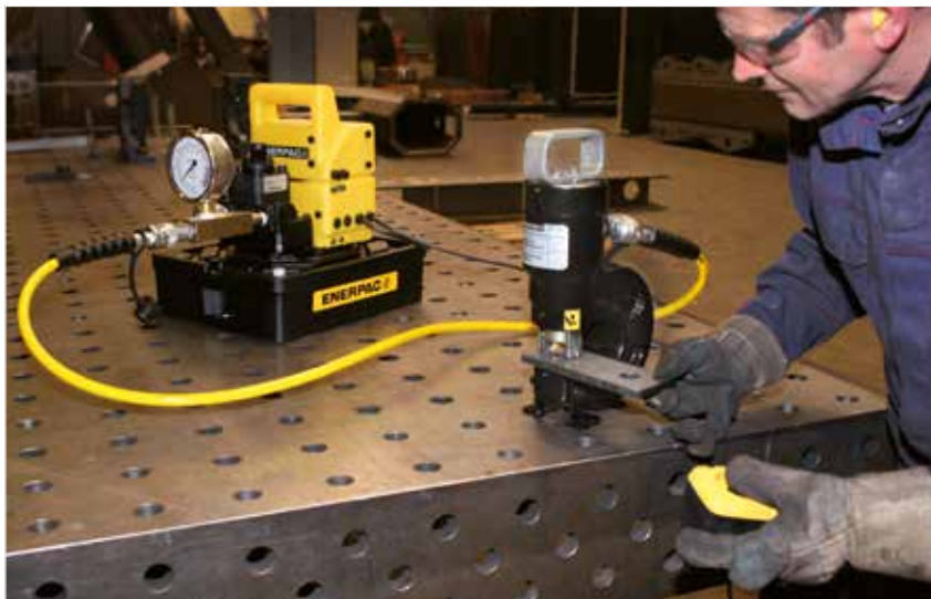
▼ SP-Series, Lightweight Hydraulic Punch – Much Faster than Drilling.
