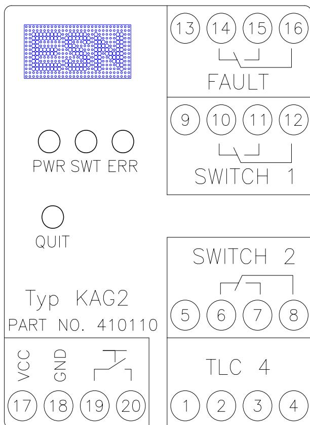
Assignment DIN rail adapter
