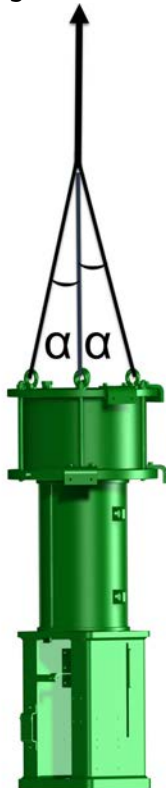
Figure 9. Lifting Angle for Welded Eyelets
