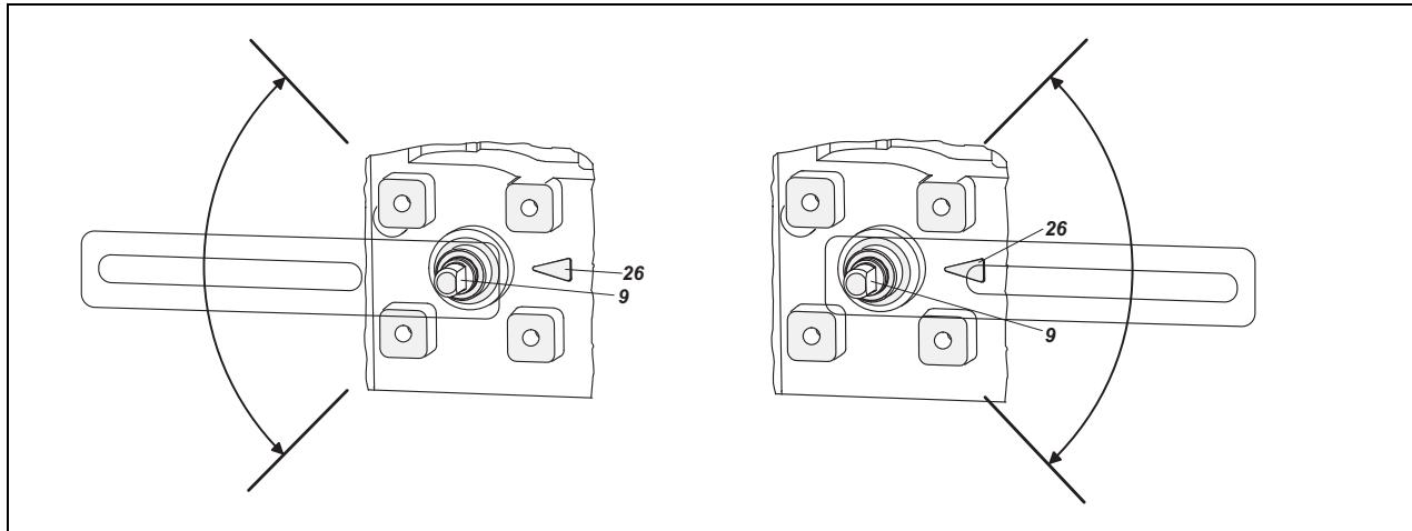
Any mechanical backlash may be source of poor control, oscillation and hunting as well as long duration of Autostart. Please use only original mounting parts and ensure that they are correctly mounted and tighten. By not using the original feedback lever or by using them in an inappropriate way, the performance of the positioner may be compromised.
