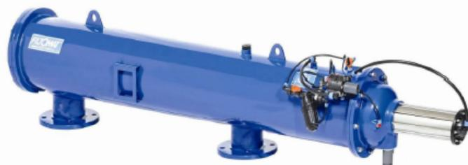
The automatic flushing cycle described below takes a few seconds and does not interrupt the supply of process water. Water flows from the inlet through the coarse and fine screens to the outlet. At a pre-set pressure differential (0.5 bar — 7 psi), the rinse controller activates the piston and opens the flushing valve. The water from the rotor chamber flows out the drain. The pressure in the rotor chamber drops, releasing a strong flushing stream that flows through the filter.
