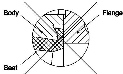
Remove the flange-spreaders and tighten the flange screws slightly and evenly crosswise with the disc fully opened.
