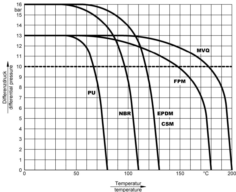
For a differential pressure of more than 13 bar valves > DN 200 have to be equipped with a seat having a higher shore hardness.
