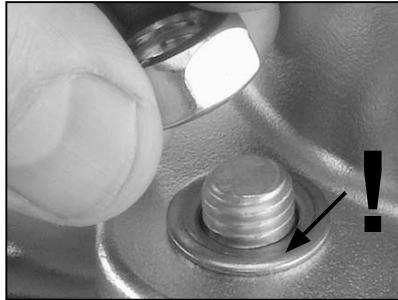
9. Insert the four bolts with their respective washers from the body side and tighten diagonally hand tight only. (Do not use force).
