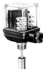
The GEMÜ 1230 electrical position indicator have one or two microswitches for end position feedback which are mechanically adjustable. GEMÜ 1230 is suitable for mounting to linear actuators with a max. stroke of 20 mm.
