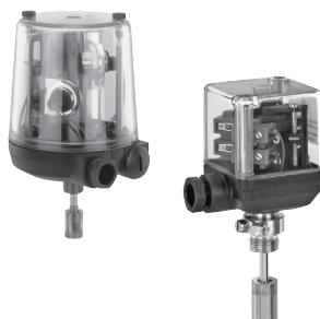
The GEMÜ 1211 and 1231 electrical position indicators have one or two proximity switches for end position feedback which are mechanically adjustable. The devices are suitable for installation in Ex-proof applications acc. to ATEX. GEMÜ 1211 is suitable for mounting to linear actuators with a max. stroke of 70 mm. GEMÜ 1231 is suitable for mounting to linear actuators with a max. stroke of 20 mm.
