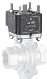
The GEMÜ 1225 electrical position indicator is suitable for mounting to quarter turn actuators of GEMÜ butterfly valves DN 15-50 mm in PVC-U, brass and stainless steel. In addition to electrical indication of end positions via switches the device has an optical LED position indication as standard.
