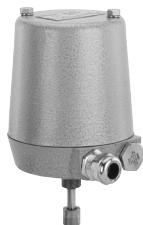
The GEMÜ 1205 electrical position indicator has one or two microswitches for end position feedback which are mechanically adjustable. The device is suitable for installation in Ex-proof applications acc. to ATEX. GEMÜ 1205 is suitable for mounting to linear actuators with a max. stroke of 70 mm.
