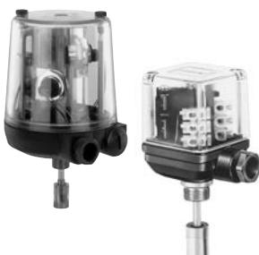
The GEMÜ 1214 and 1232 electrical position indicators have one or two proximity switches for end position feedback which are mechanically adjustable. GEMÜ 1214 is suitable for mounting to linear actuators with a max. stroke of 70 mm. GEMÜ 1232 is suitable for mounting to linear actuators with a max. stroke of 20 mm.
