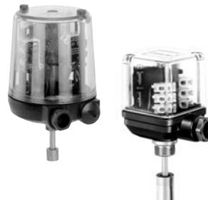
The GEMÜ 1201 and 1230 electrical position indicators have one or two microswitches for end position feedback which are mechanically adjustable. GEMÜ 1201 is suitable for mounting to linear actuators with a max. stroke of 70 mm. GEMÜ 1230 is suitable for mounting to linear actuators with a max. stroke of 20 mm.
