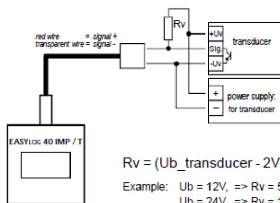
$$Rv = (Ub_{transducer} - 2V) / 2 \text{ mA}$$
