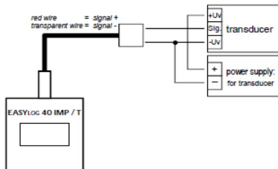
Connection example for a transducer with npn-output (e.g. FHK-PVDF):
