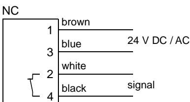
The switching outputs are self-configuring, depending on whether they are connected as PNP or NPN switches.
