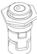
The shaft seal is screwed into the pump head.
