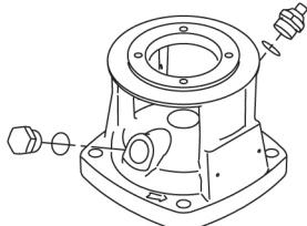
The pump is fitted with a balanced O-ring seal unit with rigid torque transmission system. This seal type is assembled in a cartridge unit which makes replacement safe and easy. Due to the balancing, this seal type is suitable for high-pressure applications. The cartridge construction also protects the pump shaft from possible wear from a dynamic O-ring between pump shaft and shaft seal.
