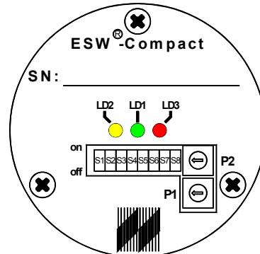
Upon execution of the self-test function, it's absolutely necessary to return the switch S8 to the position OFF in order to ensure the proper function of the ESW®-Compact-Alu. The yellow LED must darken and current has to return to his normal value. In case the yellow LED is lighting and a higher output current is flowing, without of activation of S8, than the electronic recognize one sensor defect and starts alarm, because the electronic is continuously monitoring the sensor.
