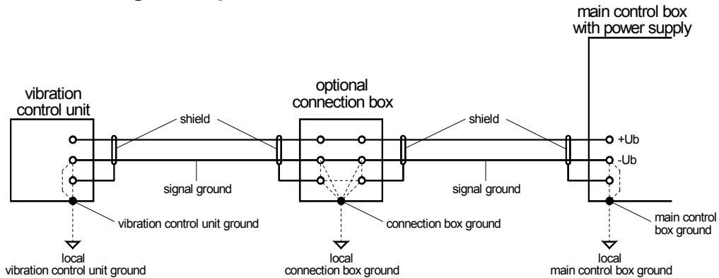
In case there is explicitly isolated installation not requested, is usually through attachment with screws each case to the local machine ground connected.
