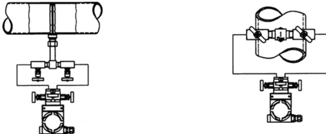
Fig. 45: Recommended sensor orientation for liquid measurement
