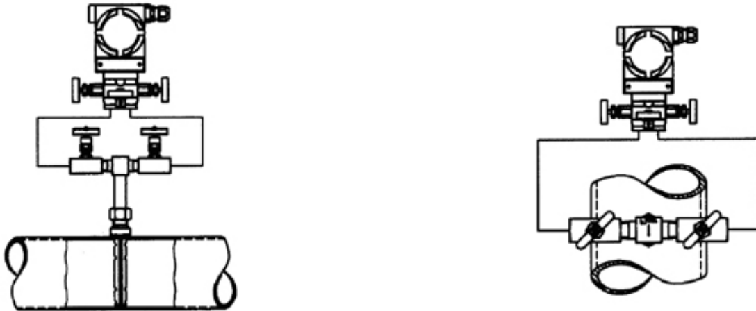
Fig. 44: Recommended orientation for measurement of gases
