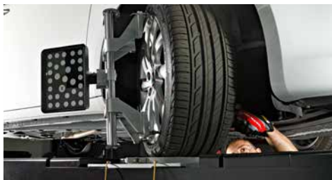
EZ-TOE for full access while adjusting front toe
