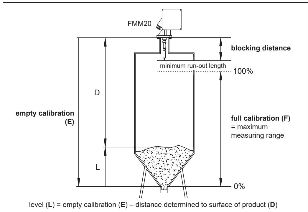
The measured value is output at the 0/4 - 20 mA current output. The sensing weight then returns to the end position whereby the measured value determined is retained until the next measurement.
