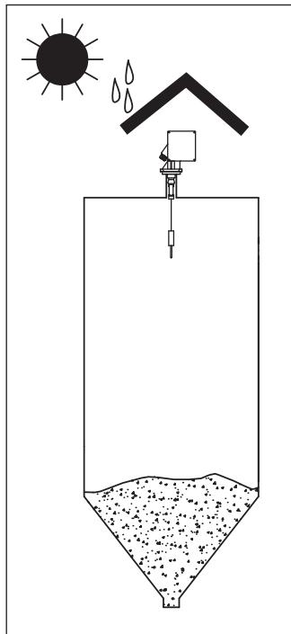
The FMM20 is best mounted on a counter flange DN100 PN16 (connection dimensions acc. to EN 1092-1) or a flange with the same connection dimensions. This counter flange must be exactly horizontal so that the FMM20 can also be mounted horizontally (maximum angle of inclination 2°).
