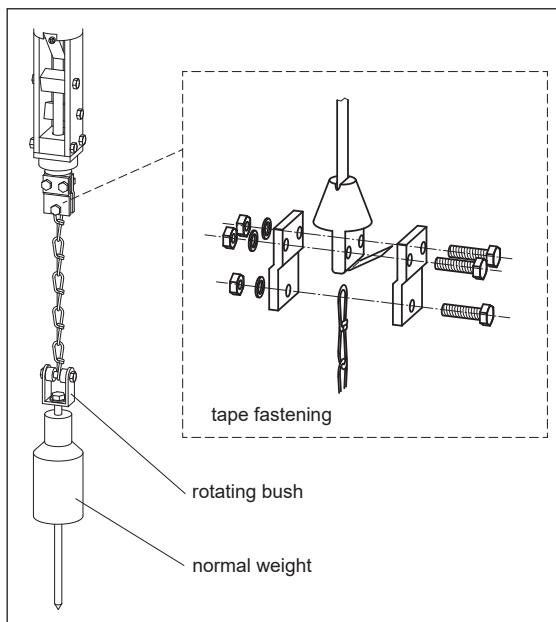
When using larger sensing weights, such as a filled medium bag for example, a point must be present in the design of the bunker or silo where these weights can be installed (see figure). Please refer to the Operating Instructions for information on mounting!
