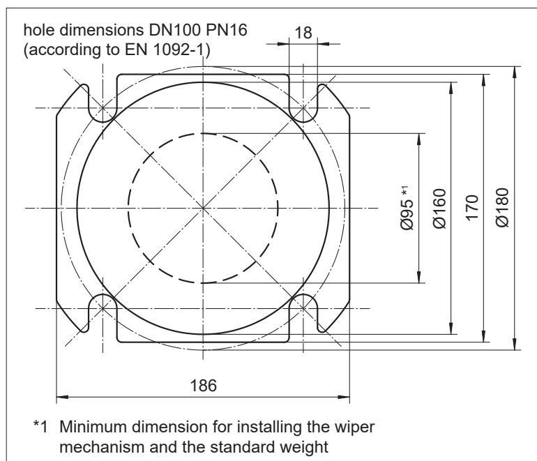
**Dimensions of the process adapter extension (accessory)**
