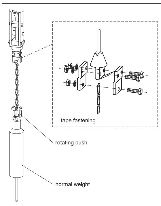
When using larger sensing weights, such as cage weights, bell weights, floats and some bag-type weights, access provision must be present in the construction of the bunker/silo for installation of these weights (see illustration). For details of these installations please refer to the operating instructions!
