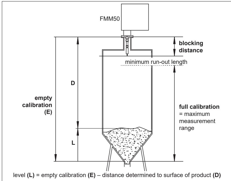
The measured value is transmitted to the 0/4 - 20 mA current output. The sensing weight now runs back up to the start position and the measured value is retained until the next measurement is performed.
