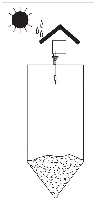
The FMM50 is best mounted on a counter flange DN100 PN16 (connection dimensions according to EN 1092-1) or a flange having the same connection dimensions.
