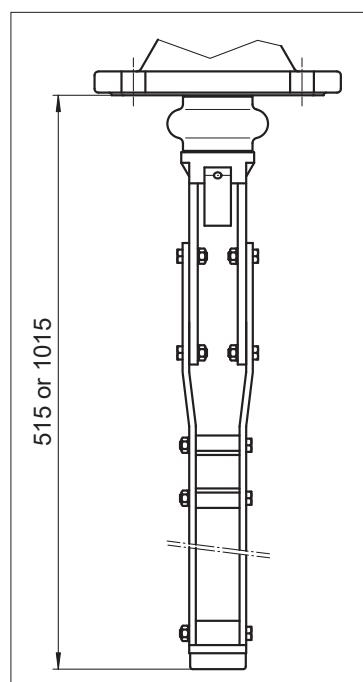
**Dimensions of the process connection (standard version)**
