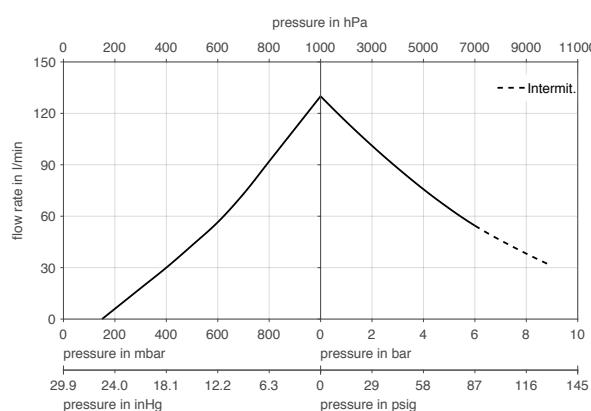
Flow rate determined at 20 °C, 1013 mbar abs.
