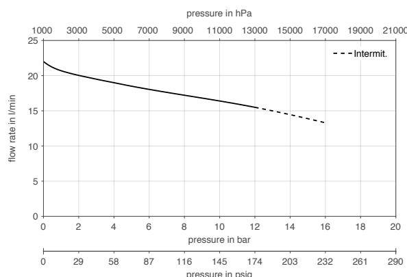
Flow rate determined at 20 °C, 1013 mbar abs.
