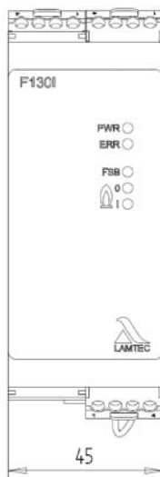
Fig. 1-2 dimensions F130I Housing material: Plastic
