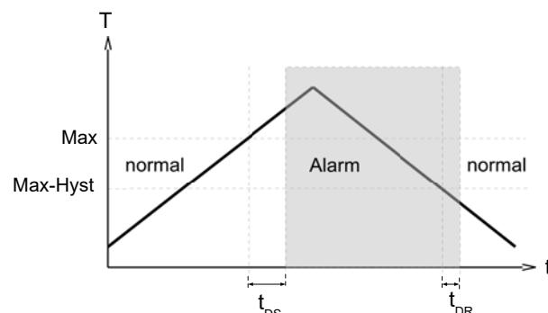
In the normal state the integrated LED is on, in the alarm state it is off, and this corresponds to its status when there is no auxiliary voltage.
