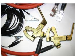
6220-756 10 m Lead set 2 x 70 mm<sup>2</sup> current leads with clamps and 2 x potential leads with clips.
