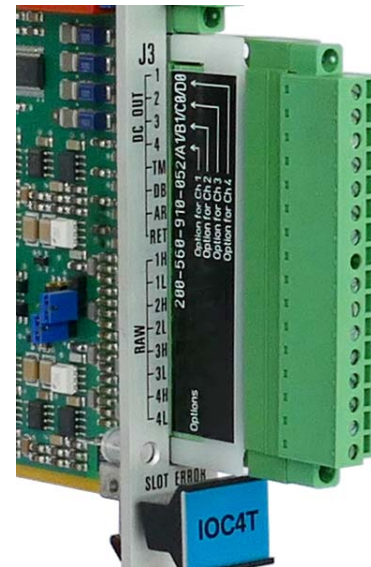
IOC 4T capacitive-coupling adaptor (shown inserted in J3)
