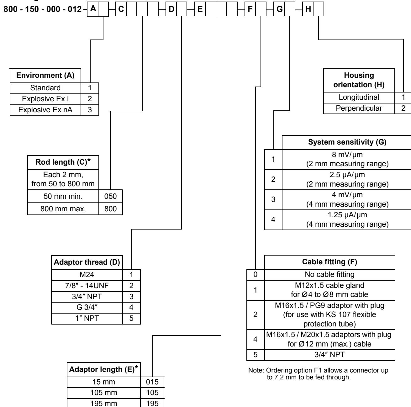
Note: Ordering option F1 allows a connector up to 7.2 mm to be fed through.
