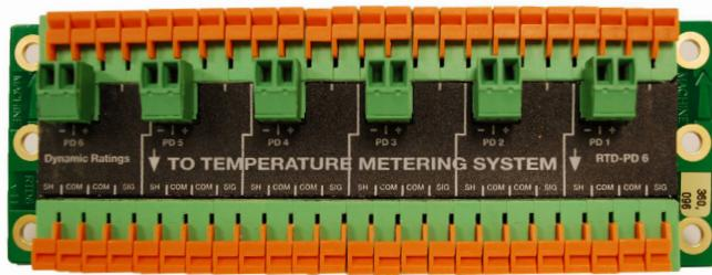
The RTD 600, from Meggitt's Vibro-Meter product line, is an interface module that enables existing RTDs (resistance temperature detectors) embedded in the windings of generators and motors to be used as additional partial discharge (PD) sensors to complement power coupling capacitors (CCs).
