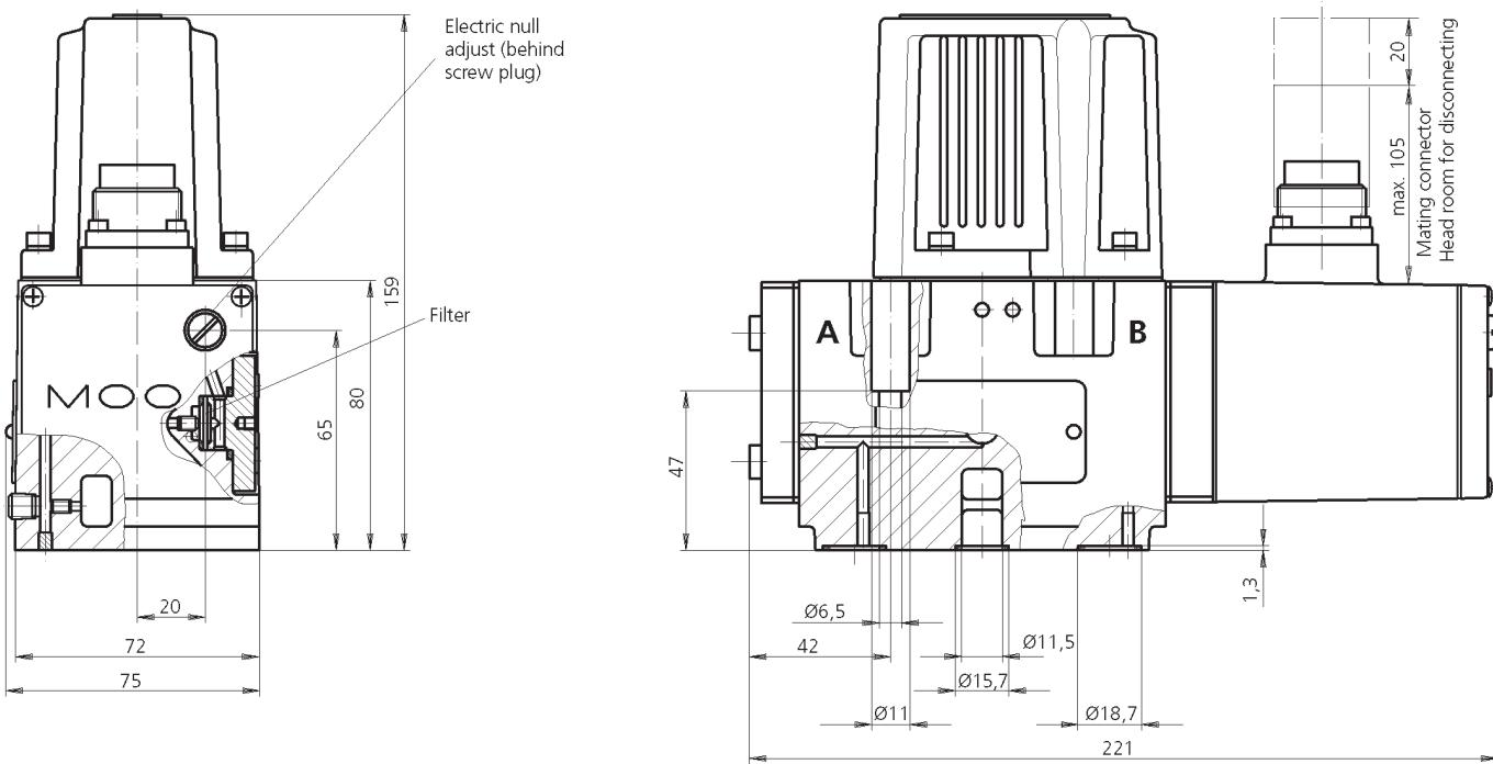
**The mounting manifold must conform to ISO 4401-05-05-0-94.**
