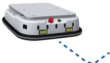
Motion Controlled with Laser (LIDAR) Sensor
