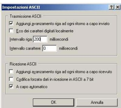
6. On the upper part of the screen ("ASCII Sending"): Enable "Send line ends with line feeds" Set "Line Delay" at 200 milliseconds
