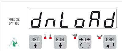
8. Press key on the DAT to start data transfer to the PC. When transfer is complete (lasting a few seconds), the instrument displays "DONE".
