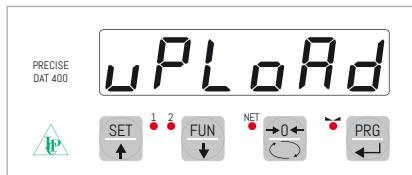
1. From the CONFIG menu, select "UPLOAD" and leave the instrument in this condition (the instrument is now ready to receive from the PC the text file containing the configuration ).
