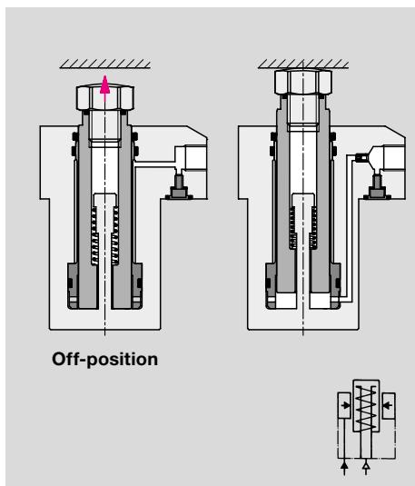
The support plunger contacts the workpiece by air pressure. The contact force is proportional to the air pressure less spring return force. The support plunger will be locked by hydraulic pressure and can compensate forces in axis direction.
