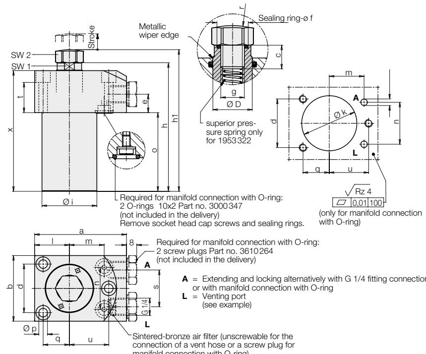
The support plunger is extended by a hydraulically pressurised small piston and contacts the workpiece with spring force.
