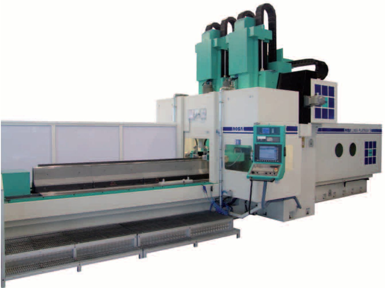
Grinding machine mod. PLATINUM TH made from Rosa Ermando SpA for MG monoguide slide ways finishing
