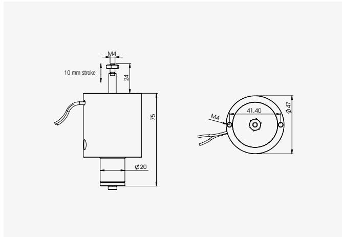
The term lifting cylinder may not be correct, however it does describe the area of application of this solenoid both simply and suitably.
