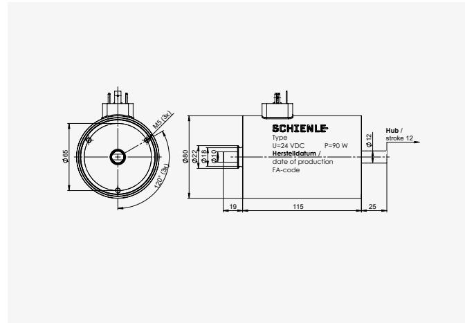
Our single-acting solenoids are available in different versions, designed for either pulling or pushing action. The plunger must be returned to its original position using external force and is operated in zero-maintenance precision bearings, ensuring a long lifetime. It is important that force is drawn off axially.
